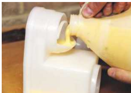
▲ The glue container is tipped on its end to allow the glue to be poured in
